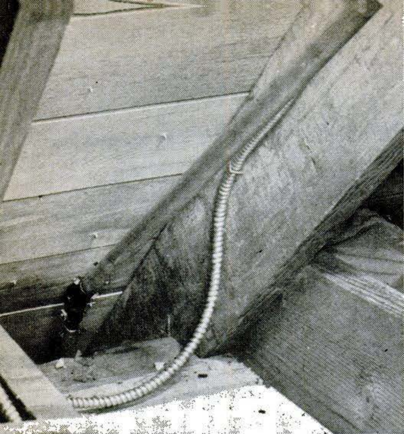
UNIVERSAL JOINT in attic links shaft to a longer drive shaft made from a TV antenna mast. Top end is bushed to fit arbor on grinder used as reduction unit.
